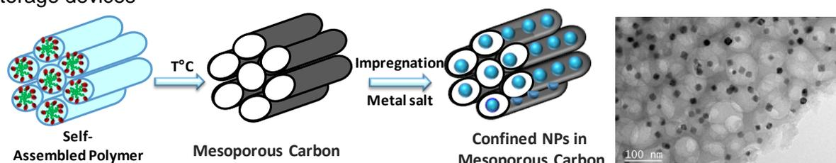
Figure 1: Schematic representation of synthesis pathway of confined metal NPs in carbon
